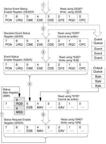
When an event occurs, a signal is sent to the DESER (1). If that type of event is enabled in the DESER (that is, if the bit for that event type is set to one), the appropriate bit in the SESR is set to one, and the event is recorded in the Event Queue (2). If the corresponding bit in the ESER is also enabled (3), then the ESB bit in the SBR is set to one (4).
