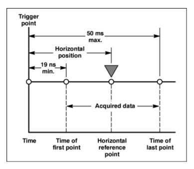
The position of the Mag timebase is constrained to be in the domain of the Main timebase. Changing the Main timebase position can affect the position of each Mag timebase, but a Mag timebase position cannot affect the Main timebase position.
